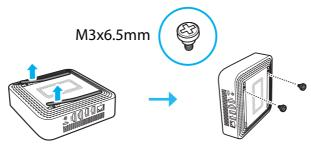
3. Align and install your Chromebox to the screw holes in the mounting plate.
