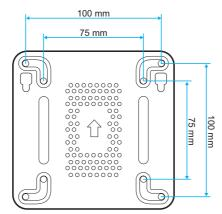
Secure the mounting plate (optional accessory) to the VESA mounting holes behind your display device with the four M4x10mm screws.
